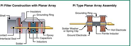
~ Built with Pi Tubes, Discoidal or Planar Arrays
