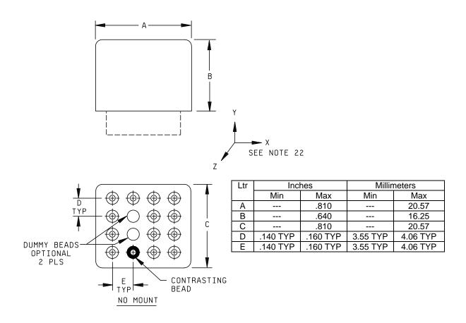
FIGURE 1. <u>Dimensions and configurations</u>.
