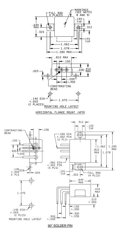
FIGURE 1. Dimensions and configurations - Continued.
