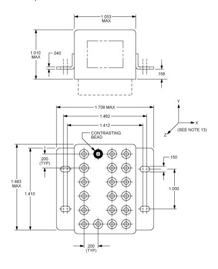
FIGURE 1. <u>Dimensions and configurations</u>.
