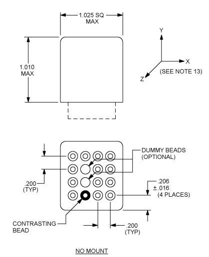
FIGURE 1. <u>Dimensions and configurations</u>.
