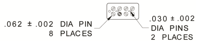
TERMINAL TYPE 2 FINISH: TIN/LEAD PLATED
