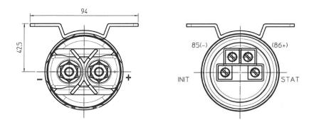
As seen in the circuit diagram (left), the important connections for control of the relay are the connections 85, 86 and INIT. The integrated electronic regulates the pulse width modulation (PWM) signal and controls the relay coil for an optimized energy usage. The STAT-output is used as an electrical auxiliary contact and can be used (for example) to analyse the amount of operating switching cycles. The STAT-output can also be used for individual customer requirements.
